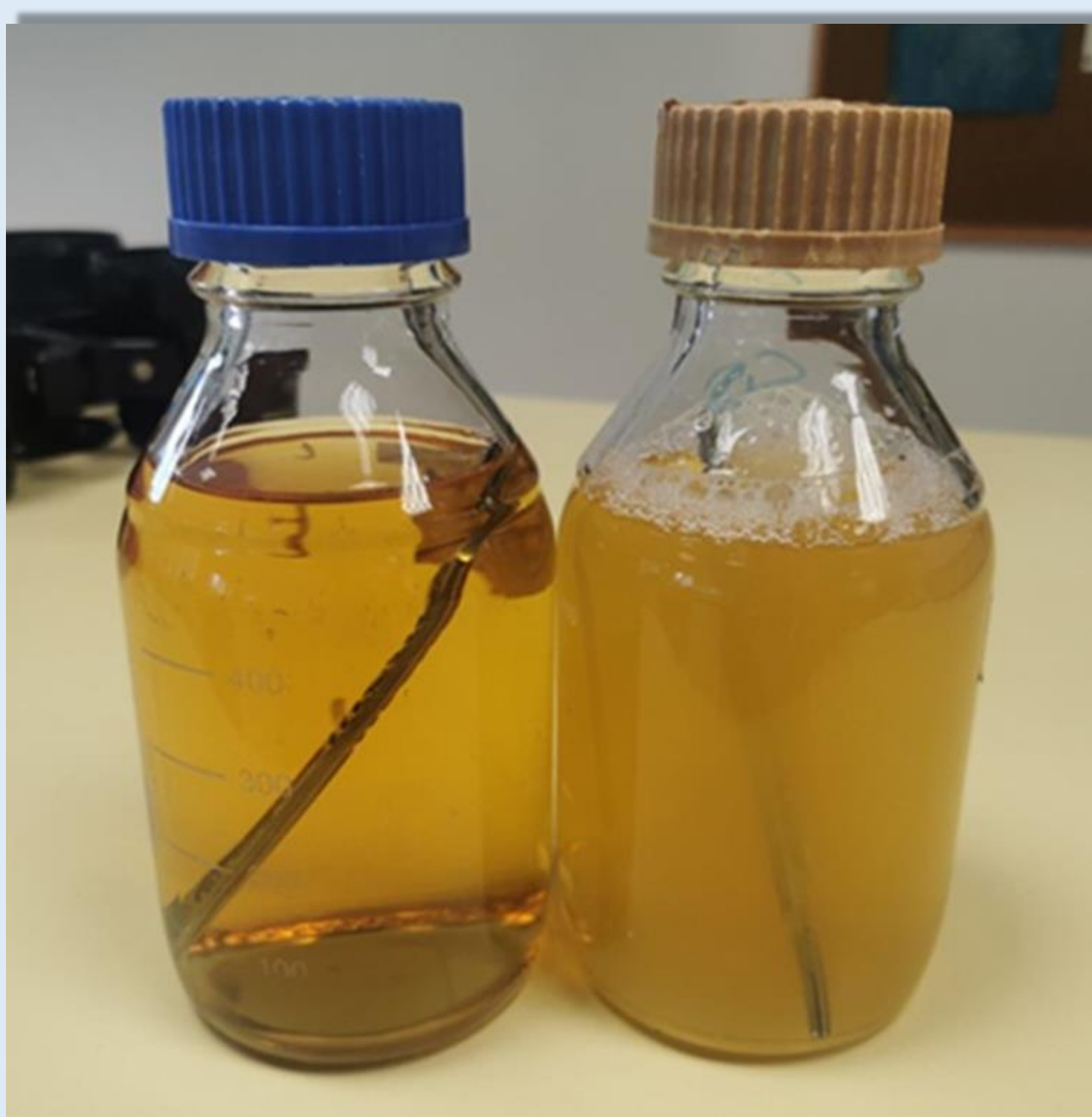
Figure 1 . Visual assessment of blade holders in NB (NB in left jar is clear, NB in right jar is cloudy/increased turbidity indicating contamination).
